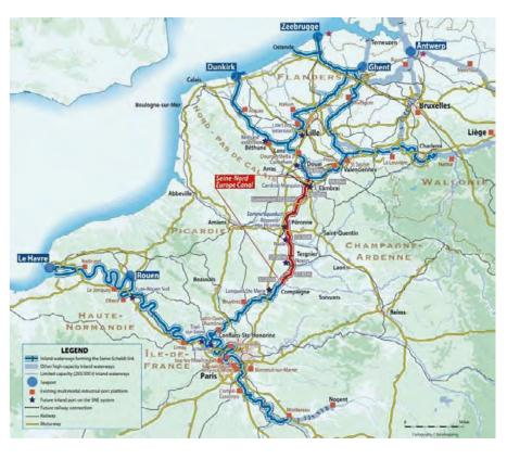
will replace the Canal de Saint-Quentin and the current Canal du Nord, increasing maximum barge capacity from 650 to 4400 tonnes.
